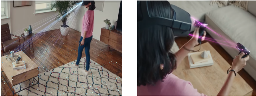
(a) The Oculus Quest headset gathering the contrast points from space. Image source: [77]. (b) The infrared light from the controllers getting tracked by the camera in the headset. Image source: [77].
