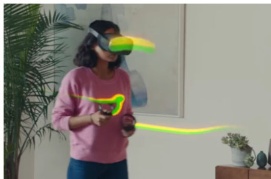
Figure 2.14: The Oculus Quest IMU's in motion, indicated by the multicolored lines. Image source: [77].
