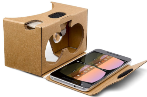
Figure 2.11: The Google Cardboard, allowing the user to insert their phone as the lens. Image source: [23].
